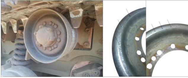
Figure 3: Merkava Mk4 Titanium track support wheel without wear ring showing less than 0.3 mm wear following a 3,000 mi field evaluation; source: Tamor SMR Ltd.
