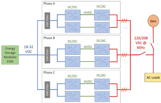
Figure 2. Power inverter box - one-line diagram.
