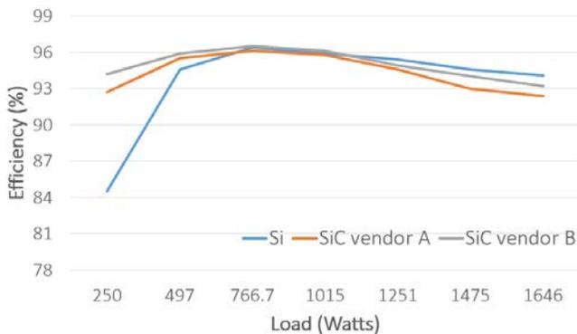
Figure 8. MOSFET Efficiency Comparison – Silicon vs. Silicon Carbide
