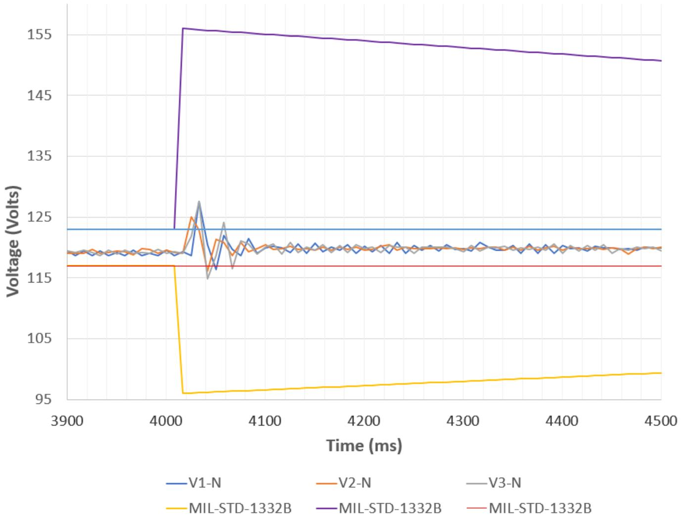
**Figure 11.** Balanced 10 kW 0.8 pf Load Step Response
