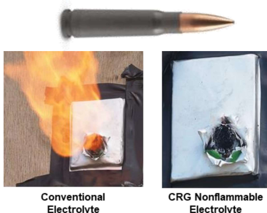
Figure 9: Ballistic penetration test, cells with conventional electrolyte versus the nonflammable electrolyte
