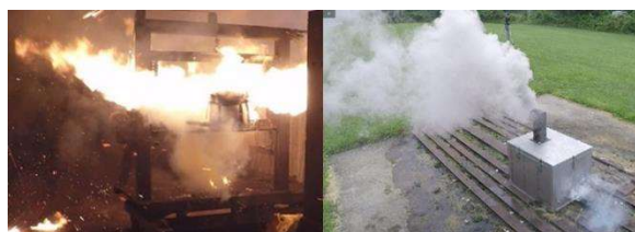
Figure 2: HSL7 battery (100% SOC) without and with a battery box, respectively
