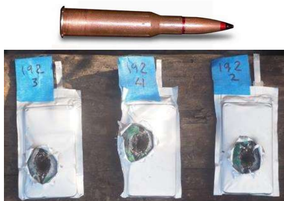
Figure 10: Incendiary tipped ballistic penetration test of the nonflammable cells
