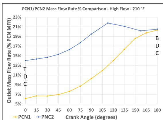
Figure 14: PCN alignment test data.
