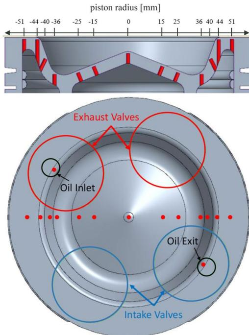
**Figure 6:** Thermocouple locations.
