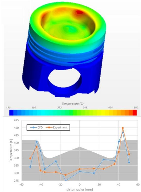
**Figure 13:** Predicted piston temperatures with Overset model.
