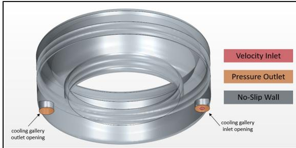
**Figure 3:** Body Force model boundary conditions.
