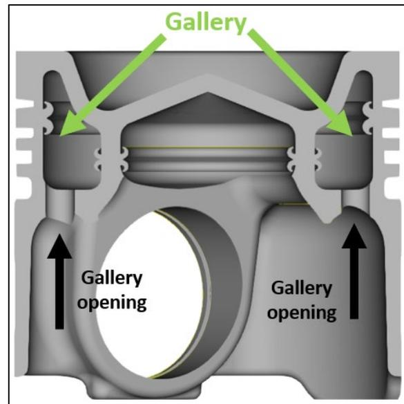
**Figure 1:** Cross section of a gallery-cooled piston.
