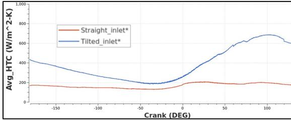
**Figure 11:** Average undercrown HTC with PCN orientation.
