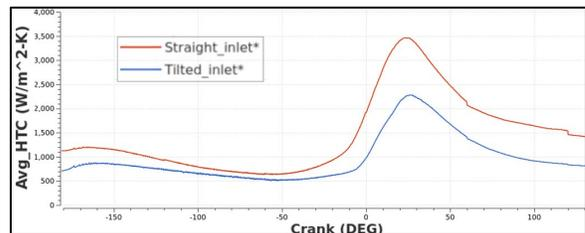
**Figure 10:** Average cooling gallery HTC with PCN orientation.
