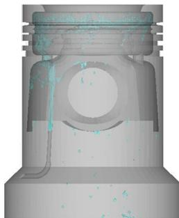
**Figure 4:** Oil flow predicted by AMR model for a misaligned PCN at piston bottom dead center.
