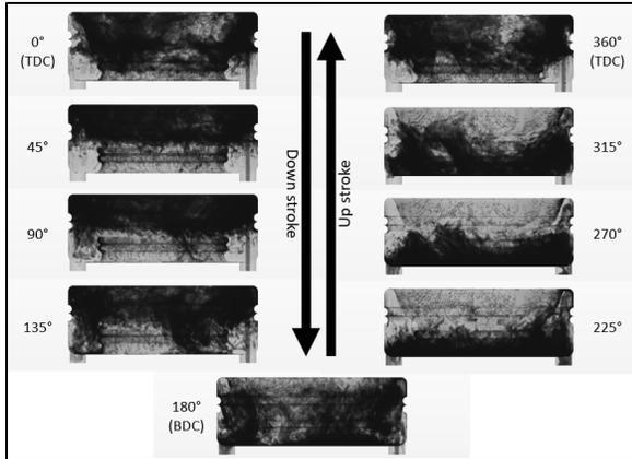
**Figure 8:** Distribution of oil within the moving piston gallery for different crank angles predicted with the Body Force model.
