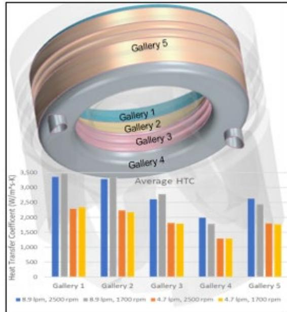
**Figure 9:** Predicted average gallery section HTC for different PCN flow rates and engine speeds.
