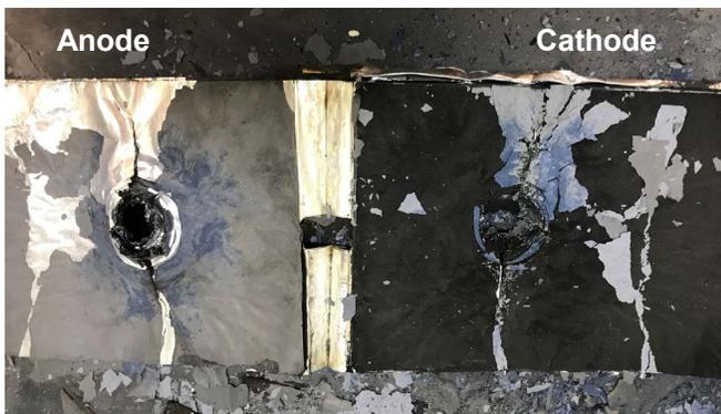
**Figure 10:** Torn down cell from 200 Wh module following penetration by 2 cm diameter nail.
