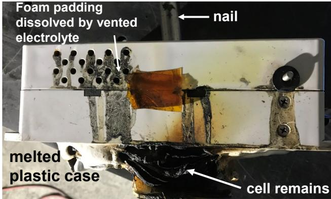
**Figure 9:** 200 Wh module after charged module was penetrated by 2 cm diameter nail.
