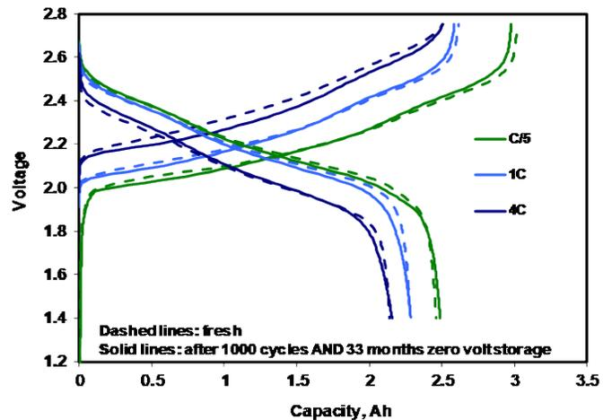
**Figure 1:** Charge and discharge voltage curves at indicated rates for a 2.5 Ah CELX-RC pouch cell before and after 1,000 full cycles at 1C/1C rate and almost 3 years storage in the 0V condition.
