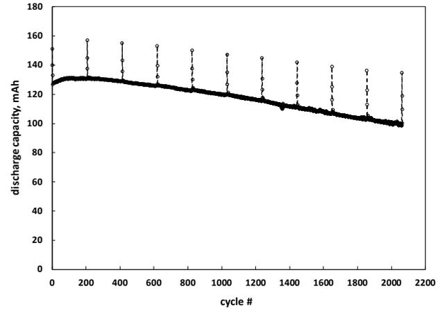
**Figure 3:** Discharge capacity of an unmanaged 11-S stack of CELX-RC pouch cells cycled 28.5 V to 20 V at 200 mA charge and discharge current, with 20, 50 and 100 mA discharges at 200-cycle intervals.
