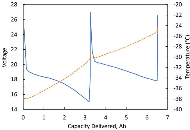
**Figure 5:** Voltage and internal temperature of CELX-RC-based 6T battery prototype at -40 °C as it was discharged at 400 A in two 30-second pulses with 5 minutes intervening rest.
