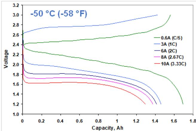
**Figure 2:** Charge and discharge voltage curves at indicated rates for a 3 Ah CELX-RC pouch cell cycled at -50 °C.
