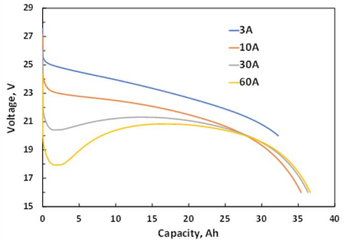
**Figure 6:** Constant current discharges of CELX-RC-based 6T battery prototype at -60 °C.
