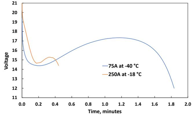
**Figure 8:** 30-second discharge pulsing at -18 °C and 75 A continuous discharge at -40 °C for CELX-RC-based 4.3 Ah battery module.
