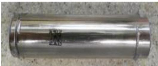
Figure 2 Tesla 2013 Model S Cell
