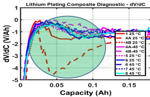
Figure 4 dV/dC of Discharge Capacity of Lithium Plating after Fast Charge Aging – Magnitude of the highlighted trough gives a Measurable Metric of Intensity of Plating
