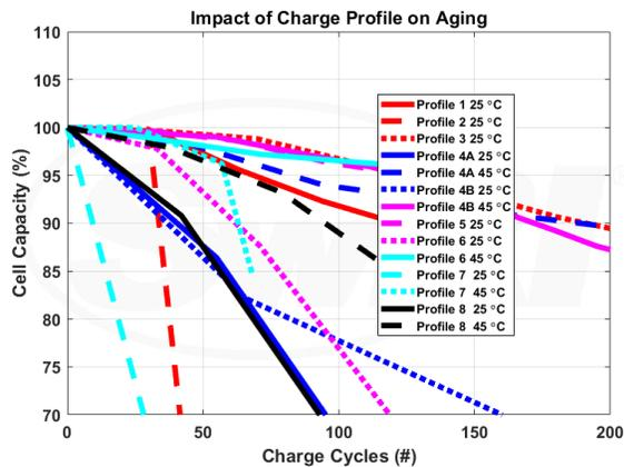
Figure 3 Degradation of capacity after multiple charge profile duty cycles
