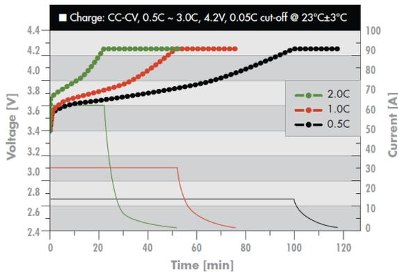
Figure 1 CC-CV Charge Protocol is most frequently Used - Courtesy: Dow Kokam/XALT
