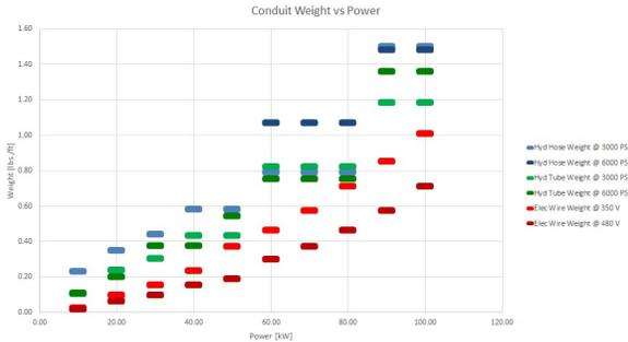
**Figure 9:** Hyd Hose, Tube and Wire Weight vs Power.
