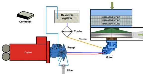
Figure 16: Cooling Fan – Hydraulic.
