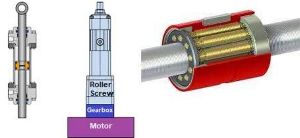
Figure 5: Elevation Actuators.<sup>17</sup>
