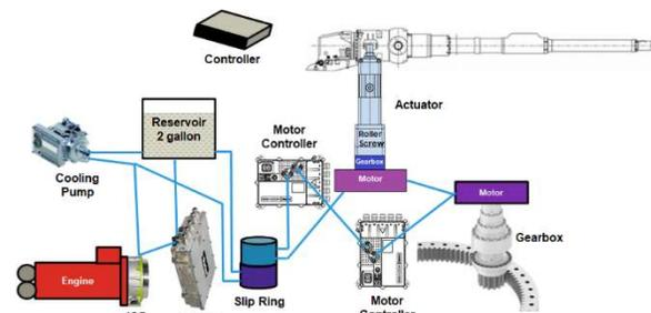
**Figure 2:** Gun Control – Electric.
