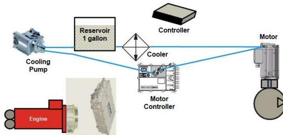
Figure 13: AC Compressor – Electric.
