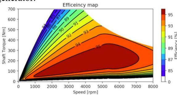
Figure 4: Typical Axial Flux Electric Motor Efficiency.<sup>6</sup>
