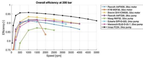
Figure 3: Typical Hydraulic Pump & Motor Efficiency.<sup>26</sup>
