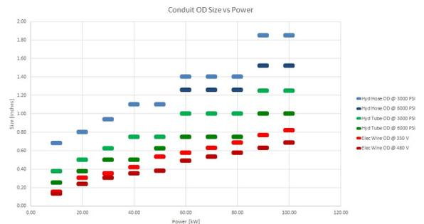
Figure 7: Hyd Hose, Tube and Wire OD vs Power.
