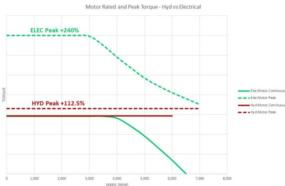
Figure 6: Motor Rated and Peak Torque. 8,29
