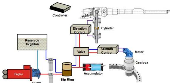
**Figure 1:** Gun Control – Hydraulic.
