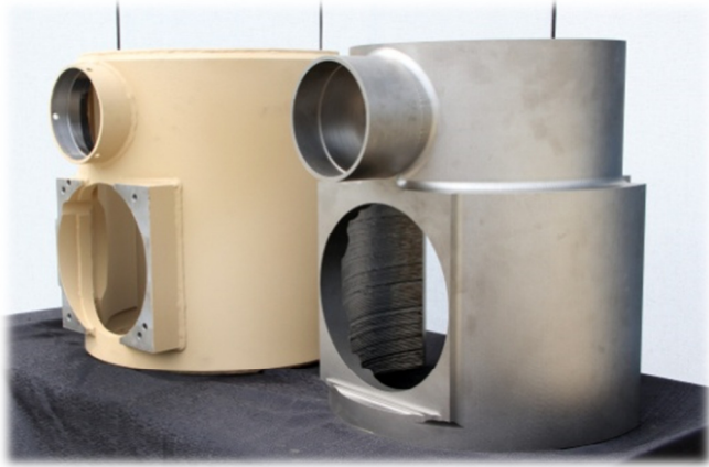
Figure B: 3D-printed titanium component (on right) with nine-piece welded steel version
