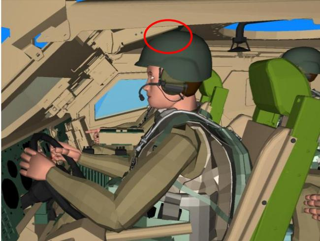
**Figure 7.** Example of encumbered boundary manikin and the impact on driver accommodation.
