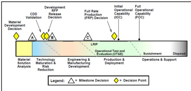
**Figure 1.** Model 1 - Hardware Intensive Program
