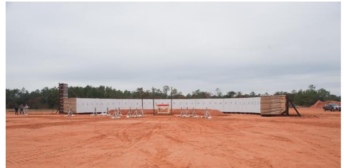
Figure 1: A weapon arena with 180° soft-catch bundles surrounding a warhead placed at the center of the arena.
