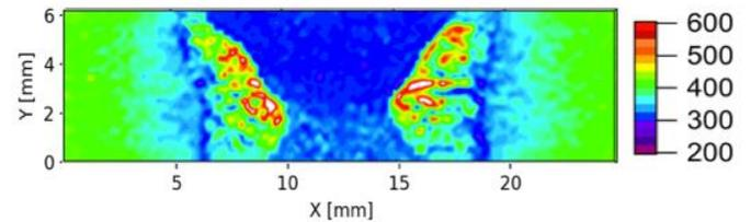
**Figure 16:** Flash® 600 single groove hardness mapping after being welded at room temp w/ ER120S-1 weld wire
