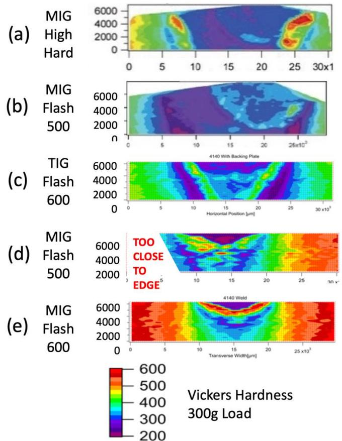
**Figure 8:** Weld hardness mapping of typical high hard (a), Flash® 500 (b & d), and Flash® 600 (c & e)
