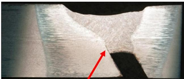
**Figure 18:** Flash® 600 Tekken y-groove sample. Note the lack of side wall fusion at the red arrow.
