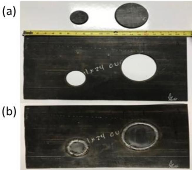
**Figure 13:** Flash® 600 welded “circles” which have been cut out (a), rotated, welded (b) without cracking
