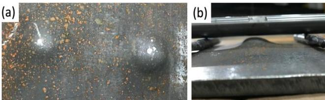
**Figure 6:** Flash® 600 back plate with 0.200" dimpling
