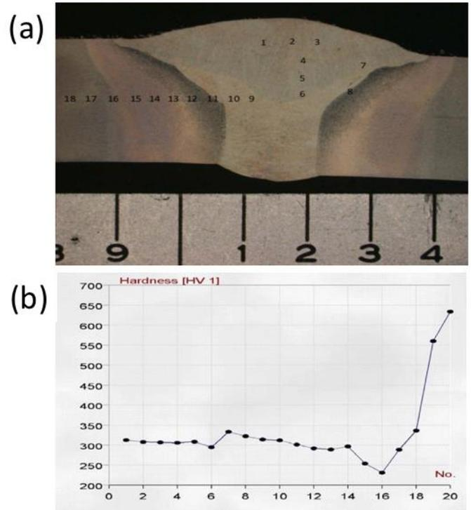
**Figure 11:** Flash® 500 HAZ showing indent location (a) with microhardness indents graphed (b).
