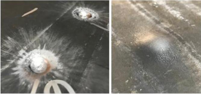
**Figure 2:** M80 ball dimples of 0.150” deep in 0.260” plate
