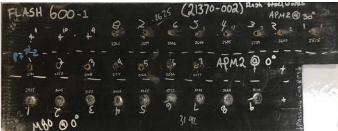
**Figure 3:** 15 shots of 0.30-cal M2AP and 9 shots of M80 ball, no cracking beyond CP perimeter
