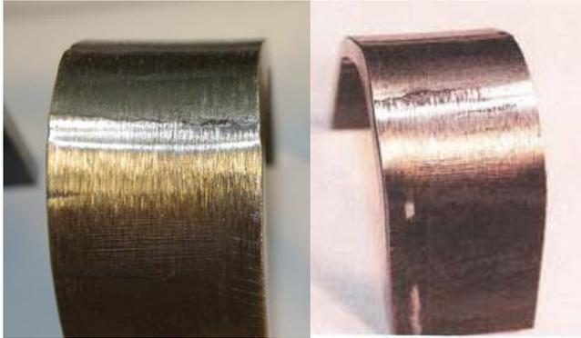
**Figure 12:** weld bends Flash® 500 (left), Flash® 600 (right)
