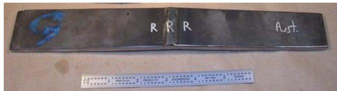
**Figure 9:** Location of three residual stress measurements on top of the plate
