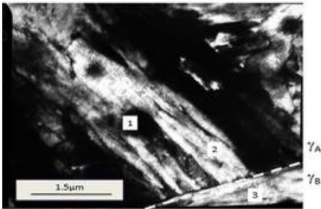
**Figure 1:** TEM showing bainitic sheaves, noted as 1, 2, and 3 in Flash microstructure. Dashed line is the grain boundary.
