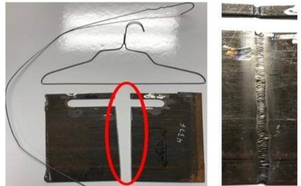
**Figure 14:** Flash® 600 butt-welded with a coat hanger at room temperature and no tempering
