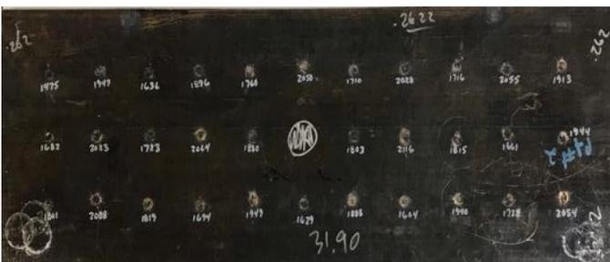
**Figure 4:** (32) PP shots of 0.30-cal M2AP at 0d, all AP cores were shattered
