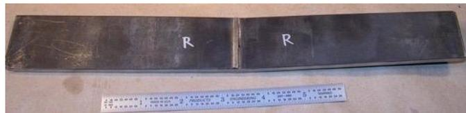
**Figure 10:** Locations of two residual stress measurements on bottom of the plate.
