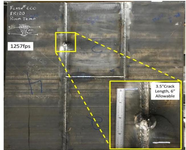
**Figure 15:** Flash® 600 butt-welded at room temp w/ ER120S-1
