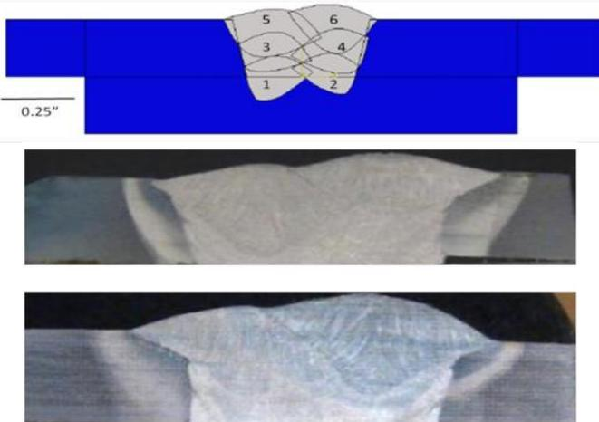
**Figure 7:** Schematic of welding used in EWI GMAW, Algoma High Hard above, Flash 500 below
