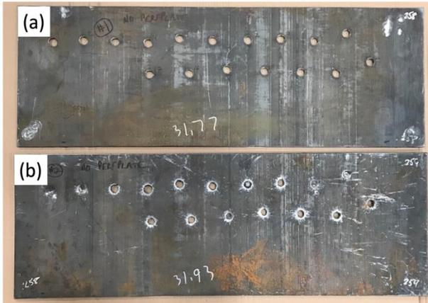
**Figure 5:** Flash® 600 strike plate (a) with (17) CPs and (11) CPs on the back plate (b)
