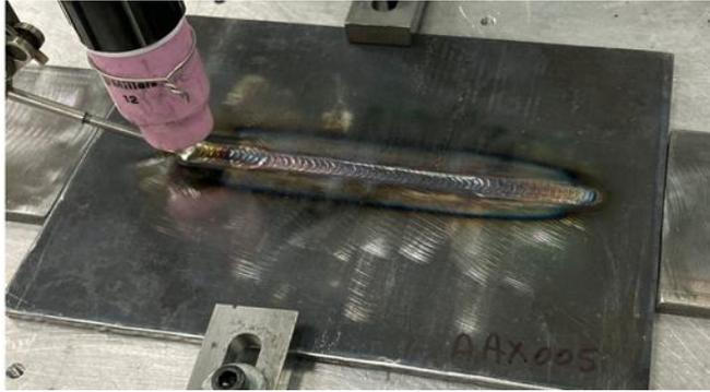
**Figure 17:** Flash® 600 Tekken y-groove sample after being welded at room temp with ER120S-1 weld wire
