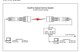
Device A can access network resources available to Device B, which can include access to the Internet. Again, both *LightSpeed* Controller Systems must be on the same subnet; also, Device A and the Router LAN port must also be on this subnet.
