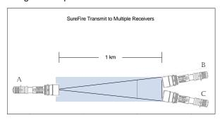
SOCS optical transmitters have a beam width of 8-10 degrees; thus, for example, at a range of 1 km, the transmit signal will cover 80 to 100m of horizontal distance. Thus it is possible for multiple units at long range to receive signal from a single transmitter, as shown in the figure above. In this scenario, units B & C receive the transmission from A, as they are both in the field-of-view of A's transmitter.
