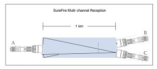
By adding multi-channel capability to the receiver, both signals could be received simultaneously. In addition, the operator at A may choose to select reception from B or C individually, using a simple rocker switch attached to the rear of the Surefire device. Please note that multi-channel capability will
