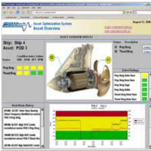
Figure 10: Acoustic based Prognostics POD monitoring software Graphic User Interface
