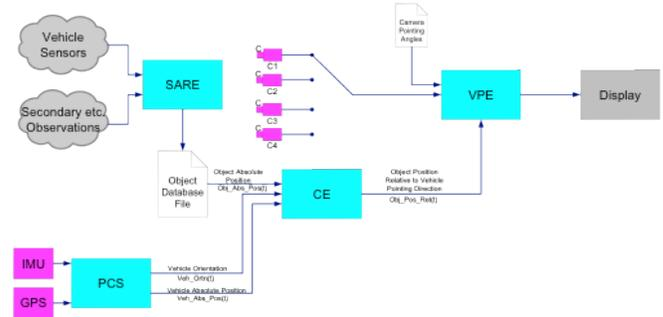
**Figure 1: Top-level System Design**
