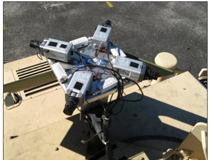
**Figure 7: Video Capture Subsystem**
