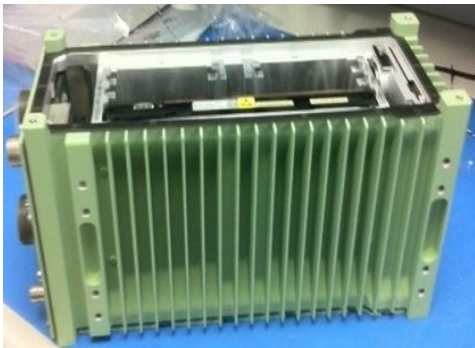
Figure 3: The 3rd generation Turret Processing Unit (TPU III) for Bradley showing hosting the VME-based Fire Control Processor and empty slots capable of hosting OpenVPX modules.
