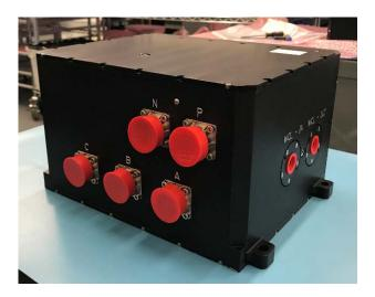
Figure 3: 75 kW SiC Based Generator Controller Hardware
