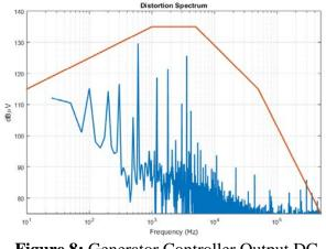
Figure 8: Generator Controller Output DC Voltage Distortion Spectrum
