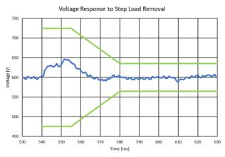
Figure 6: Generator Controller Voltage for 40 kW Load Drop Transient
