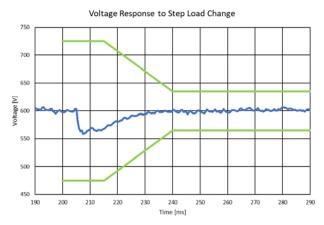
Figure 5: Generator Controller Voltage for 40 kW Step-Load Transient
