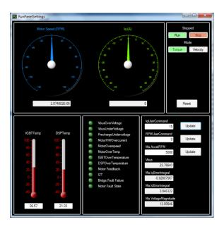
Figure 2: Generator Controller PC Interface Screenshot
