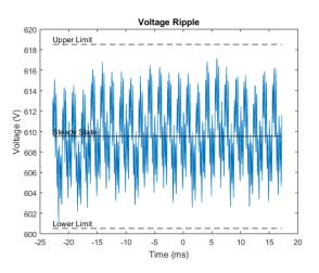
Figure 7: Generator Controller Output DC Voltage Ripple
