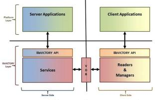
Figure 1: libVictory Software Design View [1]
