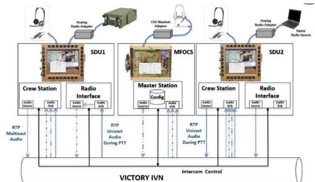
**Figure 4:** SW Intercom C4ISR Vehicle Demo Configuration
