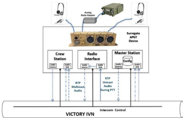
Figure 5: SW Intercom Truck Demo Configuration
